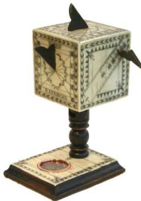
Fig. 2. Cube dial by David Beringer of Nuremberg with a direct west facing dial on its right face
