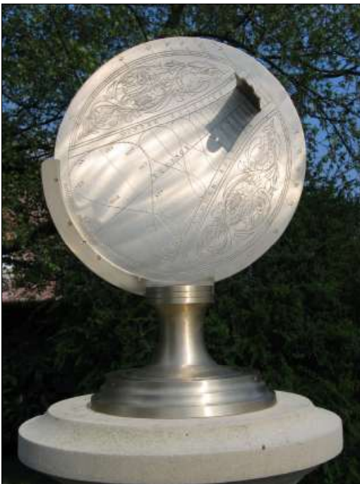
Fig. 1. The west face of a double-sided universal East/West polar dial in brass, by BSS member Harriet James.
